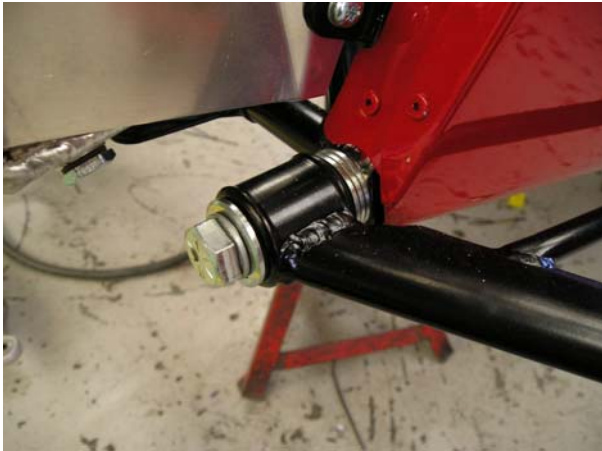
Figure 2 – Front lower wishbone assembly (front joint)
