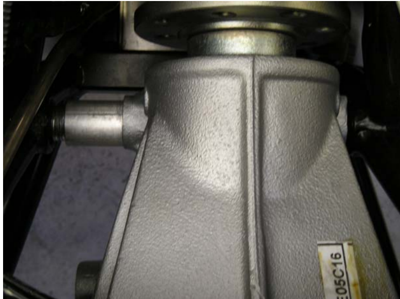
Figure 11 – Lower diff mounting spacer details
