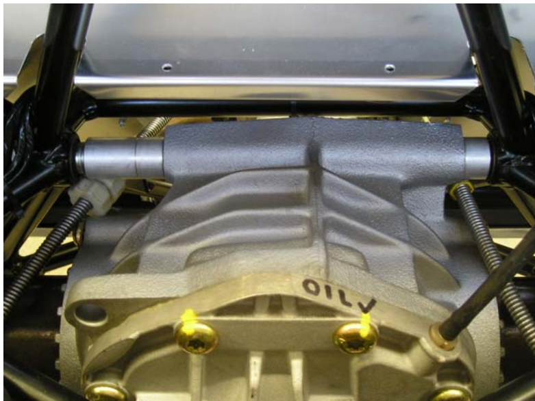
Figure 12 – Top diff mounting spacer details
