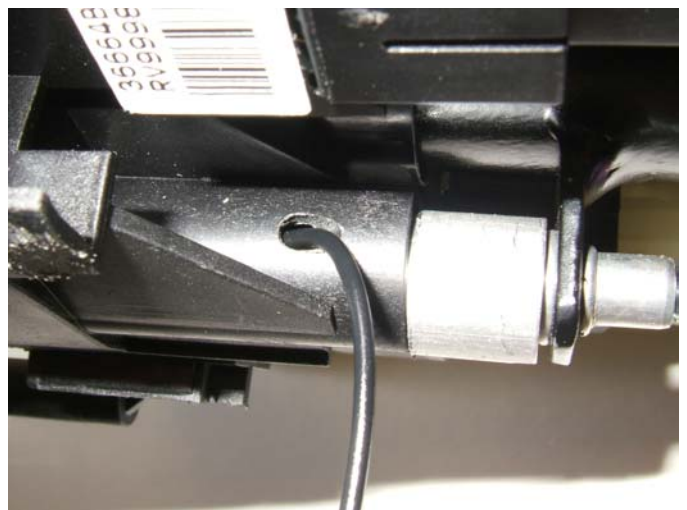
Figure 42 – Wire position for contact pin
