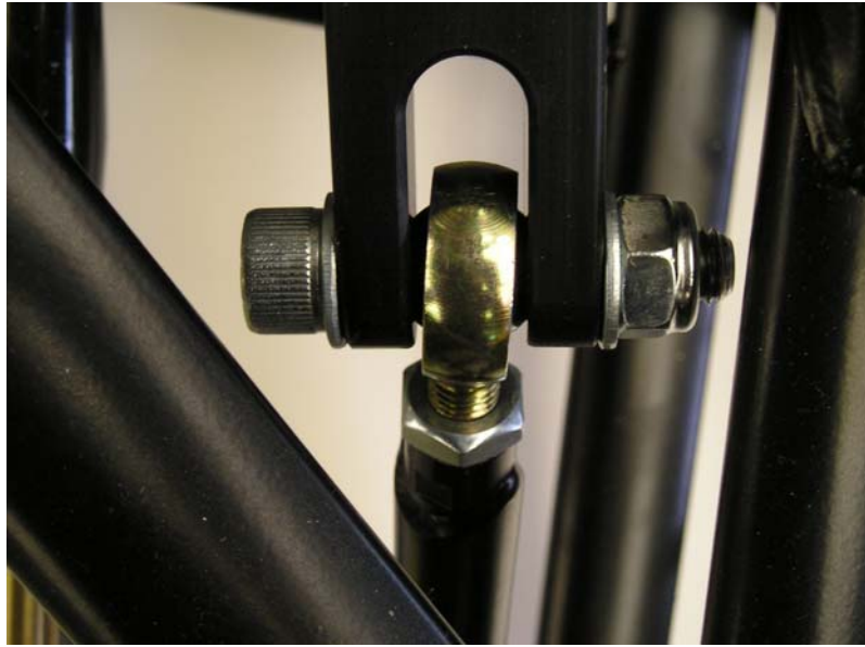
Figure 5 – Push rod to rocker joint
