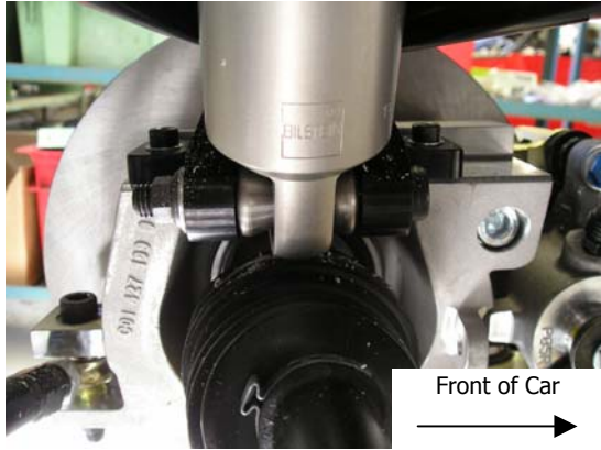
Figure 18 - Rear shock absorber to upright joint
